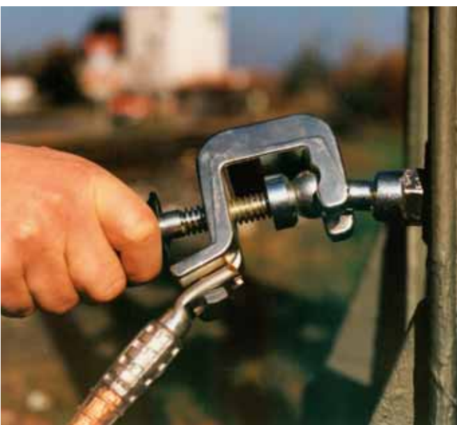
Universal earth clamp with handle connected to a fixed ball point
