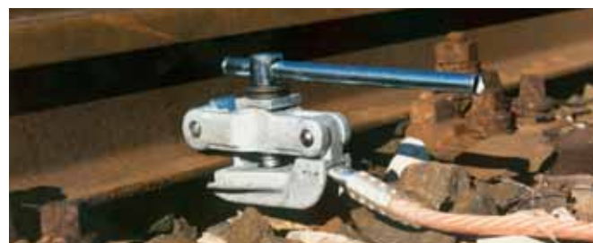
Clamp for railway tracks mounted at the track profile.
