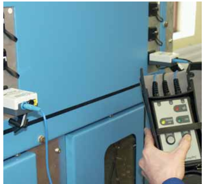
DEHNcap/PC-LRM phase comparator with two HR-LRM test adapters used in an HR switchgear installation
