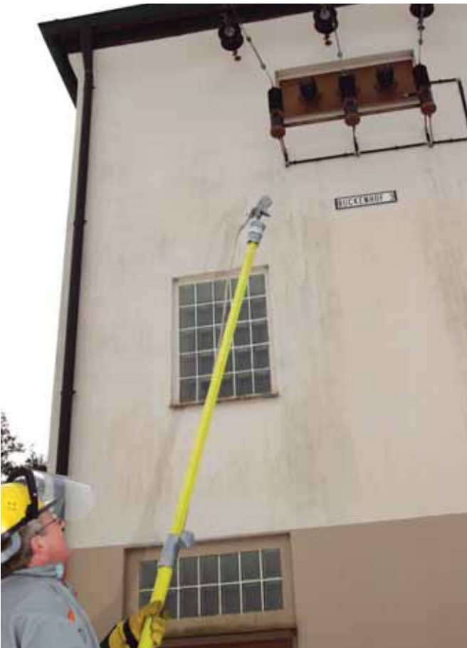
Telescopic earthing stick with aluminium cone coupling and phase screw clamp.
