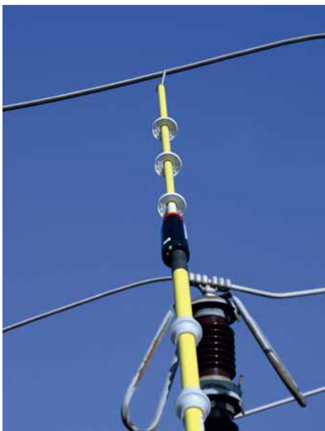
PHE III voltage detector used on a 110 kV outdoor station
